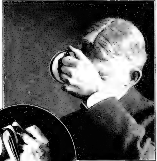
The height of a tree can be accurately measured by looking through a slot. The figures are noted on a celluloid scale as on the left
